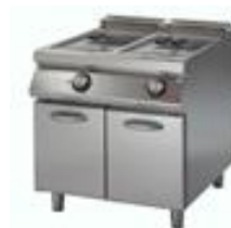
FREE STANDING DOUBLE ELECTRIC FRYER Model: 70/80 FRE17 Power: 33KW/400V Bowl capacity: 17ltr +17ltr Bowl dim: 370x250x210mm Dim: 700x800x850mm
